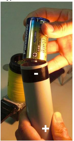
Put two UM-1 batteries. + should be connector side and - should be the lid side
