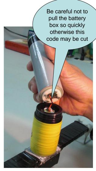
Gently take the battery case out. Do not pull too quick to prevent cutting the electric codes.
